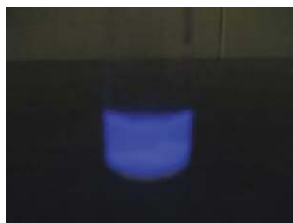
Fig. 3 The “naked eye” detection of nerve gas analog at 0.074 M concentration of DFP. A high concentration of DFP is used solely to show the glow.
